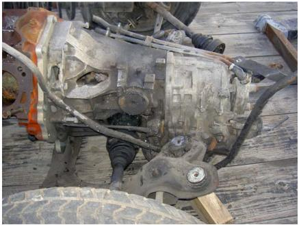
Need to remove steering linkage and axels
