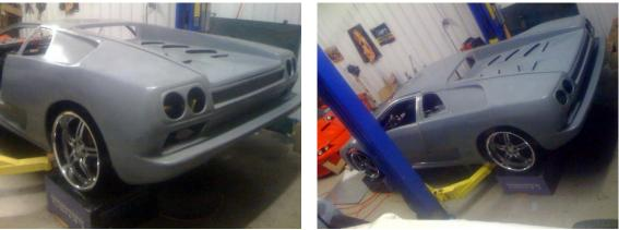
Test fitting the wheels to the project
