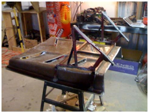
Under construction hinges . . . I'm using Iroc Z Camaro / Firebird hood hinges for my engine lid.
