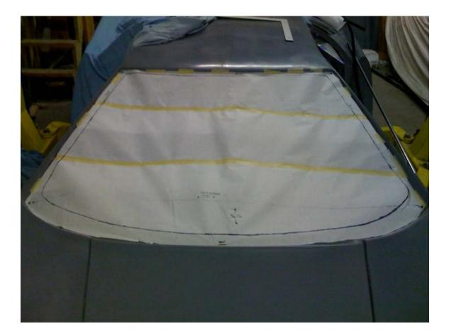
Here I show the C-channel that holds glass inside the door, for measurement reference. We need the glass to be at least to the outside black line. The inside line is what you see when window is closed. I did 2 templates. The other one has measurements and notes.
