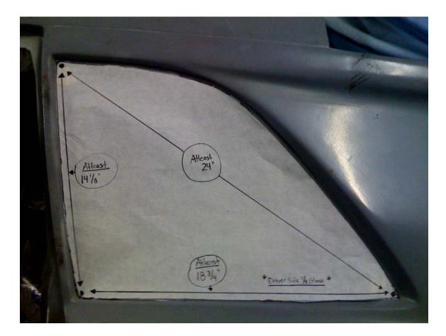
Here I cut out exactly the pattern of a windshield that would fit if the underside has same measurements as templates. Outside of glass has big curvature which will make it seem bigger in length. Underside is what bonds to vehicle. So underside is what we need to get correct. :)
