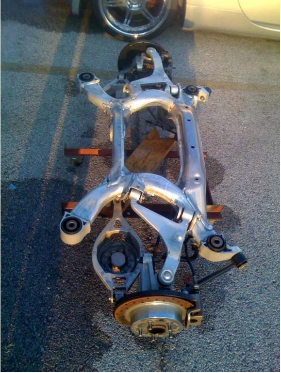
The center notch will be removed and flipped upside down to allow transaxle to sit on top.
