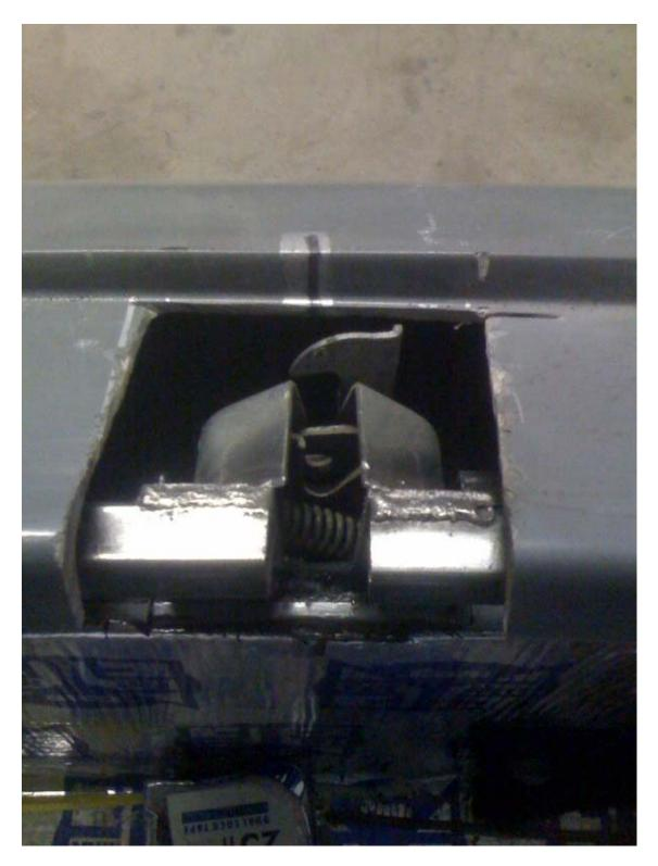
Hood latch is installed in cutaway area.
