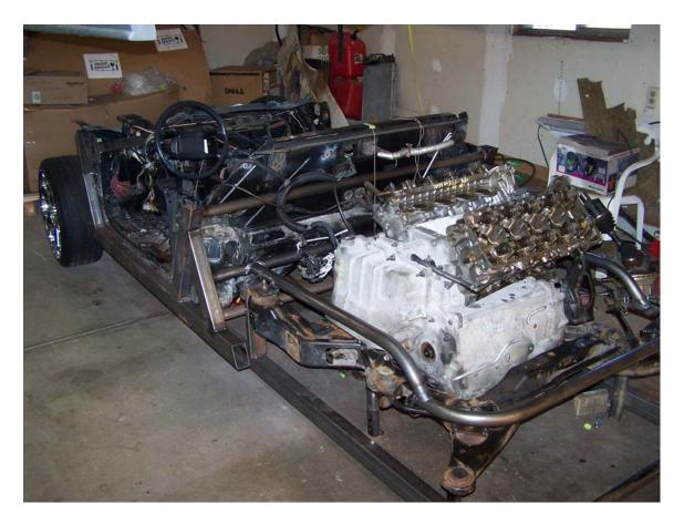
The tubing for the lower hoop has been bent and installed. The four engine cradle attachment brackets are made and welded to the lower tubing hoop. The Cadillac bare block and transmission have been installed to solve clearance problems that may or may not occur. Now I can start on modifying the Cadillac struts to accept coil overs. All measurements at this point are very critical. Measure, measure, measure.
