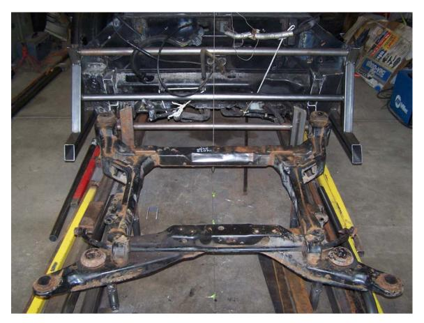
This picture shows that the two firewall cross tubing pieces have been installed, leveled, and welded in place.
