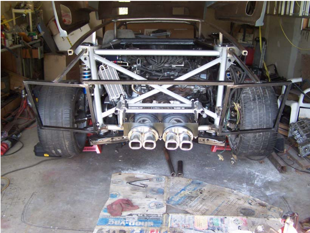
JC pic 80 - Finally got my radiator support framework welded in.
