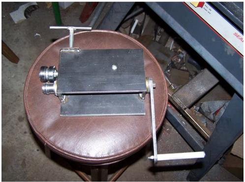
Pic 82 is the tubing bead roller that I made to bead my radiator tubing.
