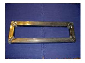
With the 1 ¼" square stock tubing, cut with 45 degree corner cuts (4) pieces 18" long (top and bottom of support/hinge frame), (2) pieces 6 ½" long on outside (front uprights), and (2) pieces 6" long on outside (rear uprights). Layout the 4 pieces for each hinge frame and weld.
