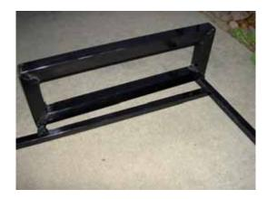
Once the rear hinge frame supports are welded under the hinge frame and butt weld to the longitudinal frame tubes, the frame can then be painted.
