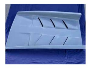
One problem with the hatch is its tendency for the front corners to curl in slightly. This requires a tubular frame to be manufactured for support and mounting of the deck lid.
