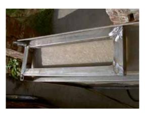
These hinge frame supports will mount to inside edge of the fiberglass deck for alignment. The bottom portion is welded to the front lateral tube of the deck frame (the end of the 2 ½" protrusion). The ¾" square by 1 ½" length tubes are welded on the longitudinal side tubes at 18" from the front edge. These will be for the rear support of the hinge frame.
