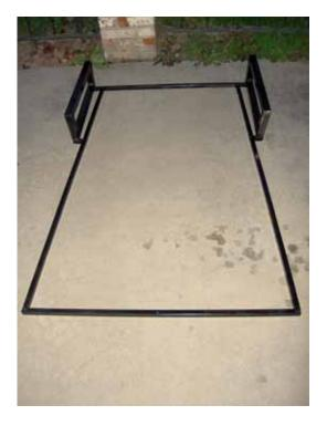
The frame consists of 3/4" X 3/4" square tubing and 1 1/4" X 1 1/4" square tubing.
