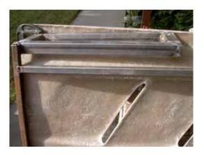
A "dry fit" is recommended after tack welding the pieces in place. The frame also needs to be checked for symmetry and square.
