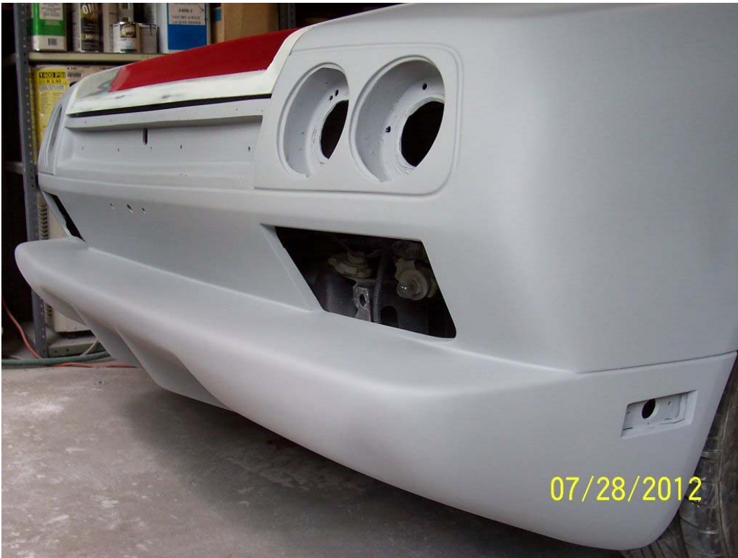
Taillight bezels installed
