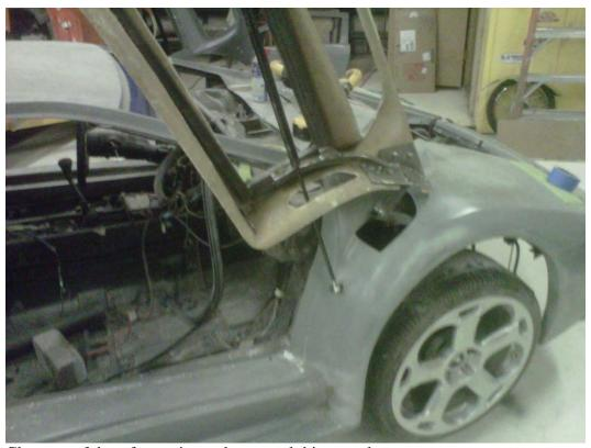
Close-up of door frame, inner door panel, hinge and strut
