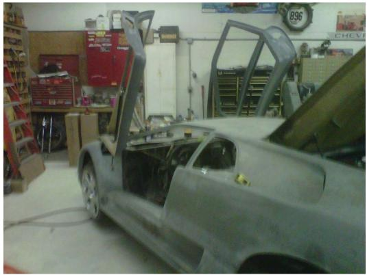
Hinges and struts installed
