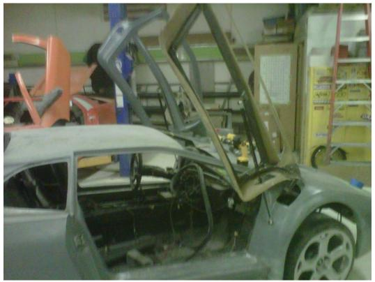
Inner door panel and frame installed
