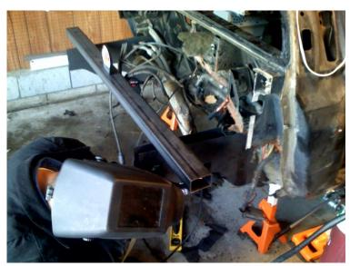
Rear of chassis/frame has been cut and removed.
