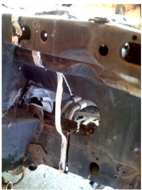
Masking tape that marked the line to cut the chassis, just like the instructions in B and B Customs article.
