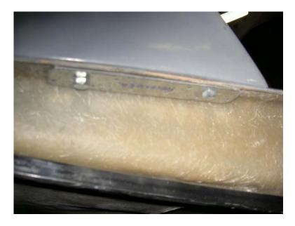
Tightening down the bolts, we have the wing installed properly.
