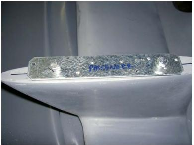
Next we fabricate two metal 1" strips approximately 7" to 8" in length. Our metal strips we used were the type used on securing boards together in construction, but you can use whatever is affordable and available. If templates were created earlier for the pilot holes in the vertical struts, they may be used to properly position the 3/8" holes. The metal strips can also be held in place under the engine hatch lips, and the holes can be marked from above the hatch.
