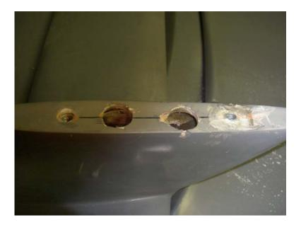
Once the T-nuts have been inserted and have epoxy or fiberglass to secure them, and have dried in position, the threads can be chased out with a tap to make sure the threads are clean and the 3/8" bolts can be tried in the T-nuts to see ease of installing.
