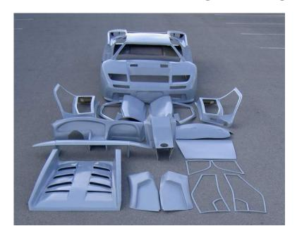
After the shock of seeing all the parts, and attaching the rear engine hatch to the chassis and body, we next can proceed with attaching the rear Wing. Actually the wing can also be attached to the engine hatch before installing the hatch, but it was felt that handling and installing of the hatch would be easier without the wing installed.
