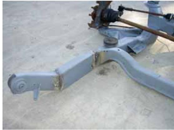
If all alignment is proper, securely weld the cradle extension tubes in place.
