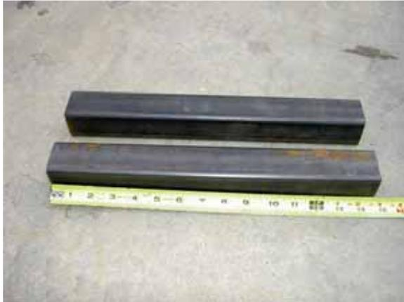
Use square tubing to extend the frame rails. Top= $1\frac{3}{4}$ " x  $1\frac{3}{4}$ " x  $14\frac{1}{2}$ " in length / Bottom=(2)  $1\frac{3}{4}$ " x  $1\frac{3}{4}$ " x  $14\frac{1}{2}$ " in length with 1/8" wall thickness (F355 uses Top = $1\frac{1}{2}$ " x 2" x 7" in length / Bottom= (2)  $1\frac{1}{2}$ " x 2" x 7"). The bottom frame rail requires two pieces of square tubing stacked one on top of the other for added stability.
