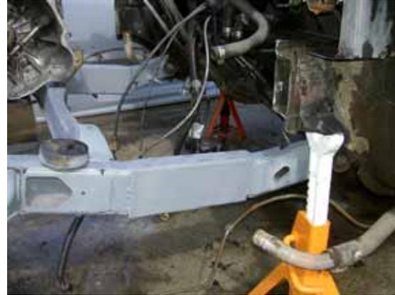
The cradle should be put on jack stands and leveled. The level can be placed on the cradle extension tubes. Using a hydraulic jack under the rear of the swing arm allows minor movements to level it.
