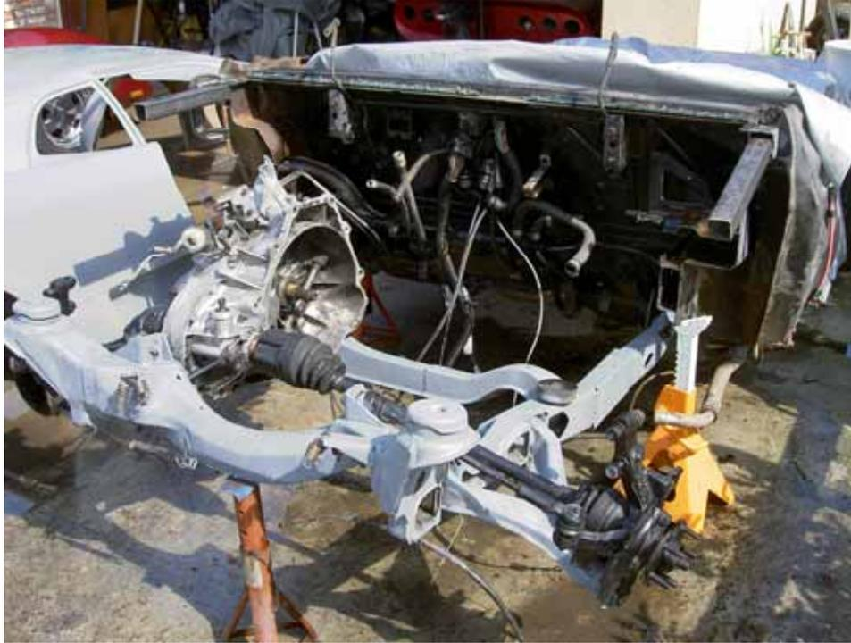
Once the upper extension tubes have been tack welded in place, the cradle should be remounted to assist with proper alignment and clearance.
