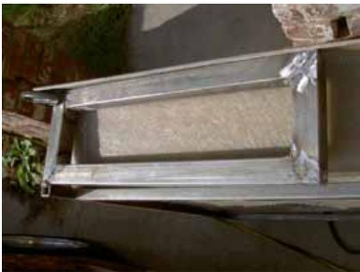
These hinge frame supports will mount to inside edge of the fiberglass deck for alignment. The bottom portion is welded to the front lateral tube of the deck frame (the end of the 2 ½” protrusion). The ¾” square by 1 ½” length tubes are welded on the longitudinal side tubes at 18” from the front edge. These will be for the rear support of the hinge frame.
