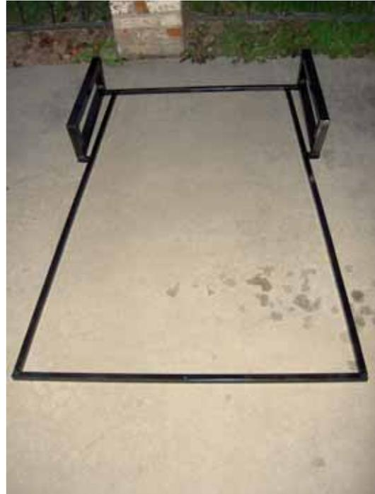
The frame consists of  $\frac{3}{4}$ " X  $\frac{3}{4}$ " square tubing and  $1\frac{1}{4}$ " X  $1\frac{1}{4}$ " square tubing.
