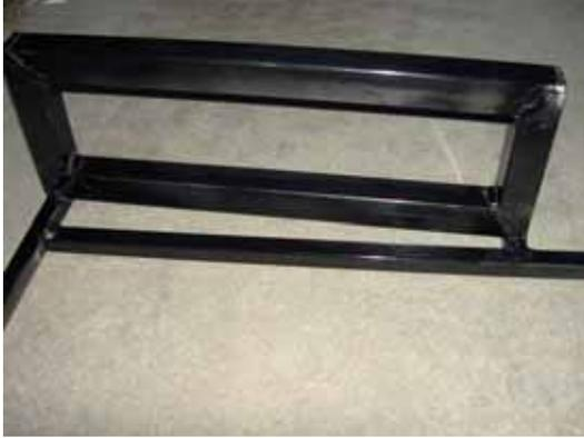
Note the 2 1/2" extension of the front lateral frame tube and the 1 1/2" rear hinge frame supports welded in place. The outer edge of these tubes are welded underneath and flush with the outside edge of the hinge frame.
