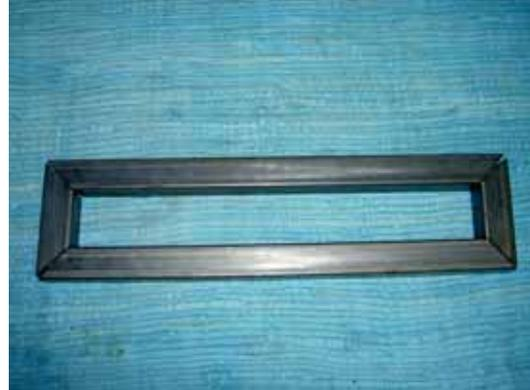
The lateral tubes are 1 1/4" X 1 1/4" square tube cut off at a 45 degree angle with 18" on the outside edge. The vertical tubes for the bottom hinge mount are 1 1/4" X 1 1/4" tubes 4 1/4" long on the outside of the 45 degree cuts. When the 4 tubes are welded together, they form a 4 1/4" by 18" boxed frame as shown in the above picture.
