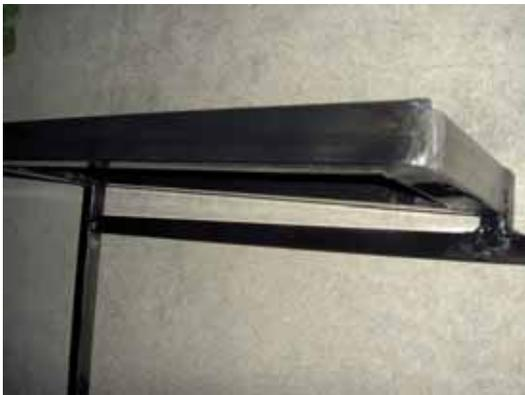
Looking from the top view, you can see the longitudinal frame tubes move outward from each other (29" apart in the front and 37" apart in the rear).
