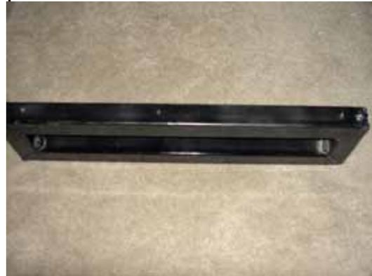
The bottom support brackets are drilled with mounting holes for securing the hinges. These 13/64" holes are at 1 3/8", 10 1/4", and 17" from the front end of the mount, with an additional 5/16" hole drilled at 1/2" for the bumper stop screw that protrudes from the bottom of the hinge arm.
