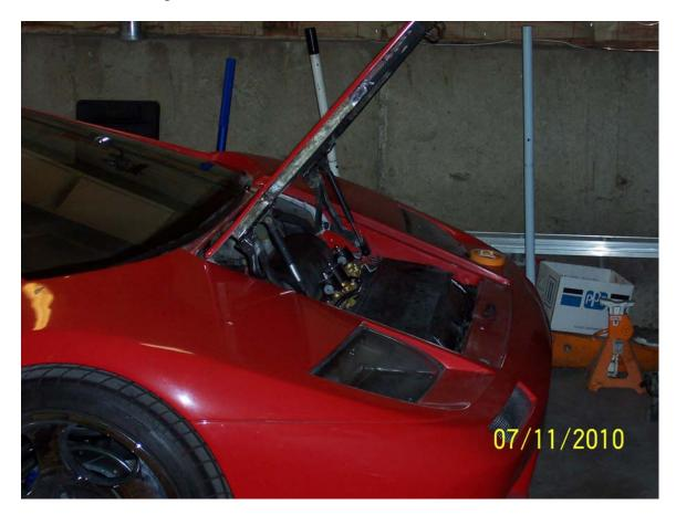
Installed new hood hinges which opens the hood away from the windshield and won't interfere with the wiper.
