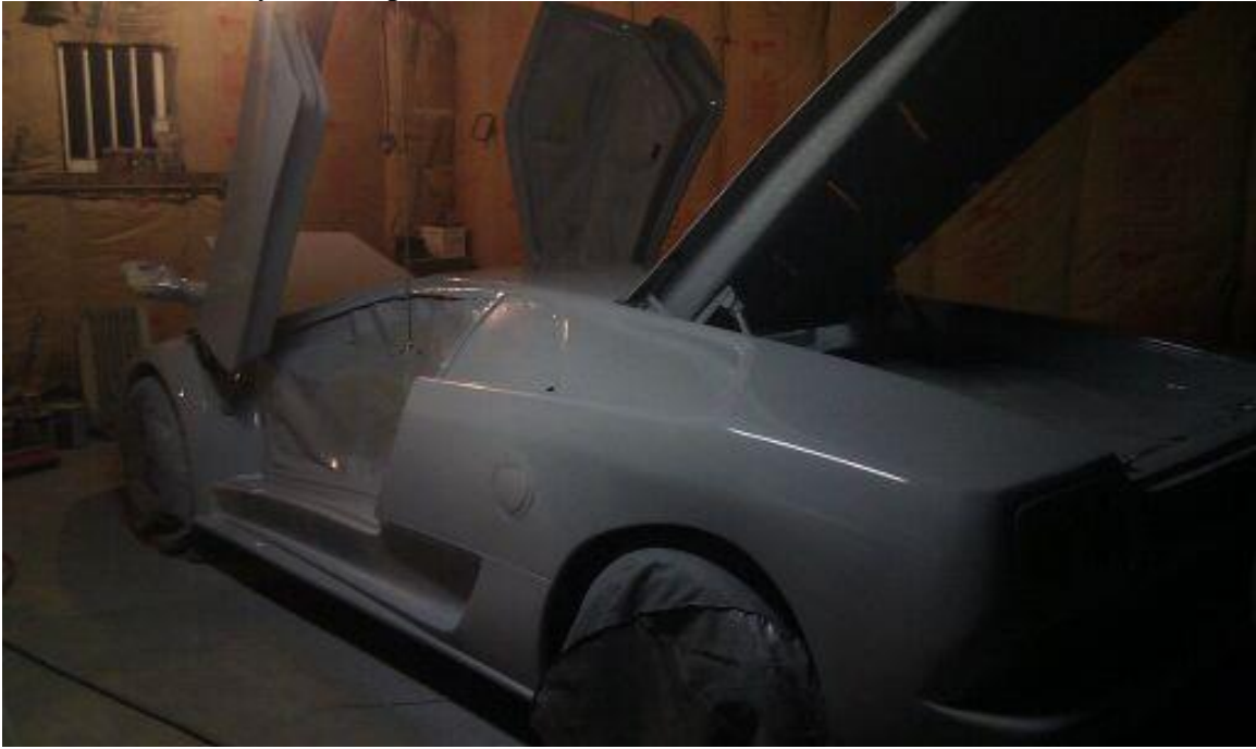
Primered and ready to start paint
